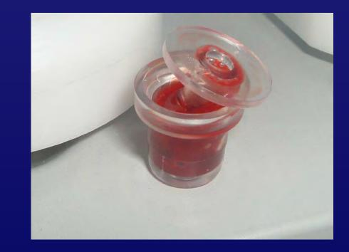
Cup rotates pin is stationary
